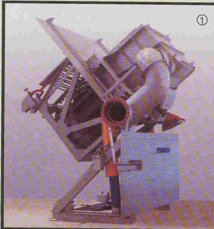
1. Coreless Induction Furnace
